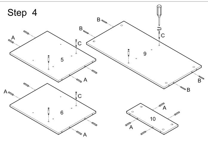
Insert dowels (B) into panel (9). Insert dowels (A) into panels (5,6,10). Screw cam bolts (C) into panels (5,6,9,10).
